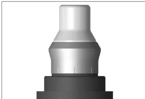
*Correct installation of insert*
