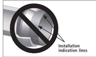
Incorrect installation of insert
