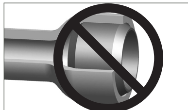
Incorrect installation of insert
