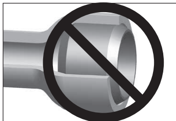
Incorrect installation of insert
