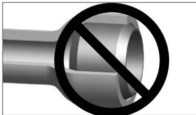
Incorrect installation of insert
